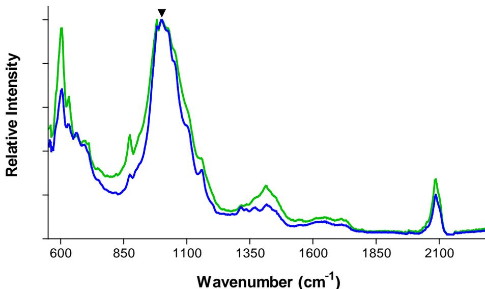
FTIR spectrum in the fingerprint region of the blue-inked portion of the PSAG-585693 stamp (blue trace) showing the equivalence in spectrum with that of the blue-inked region from the **C23c** reference spectrum (green trace). The diagnostic ultramarine peak at 1001 wavenumbers characteristic of the C23c stamp is marked with the solid wedge symbol.
