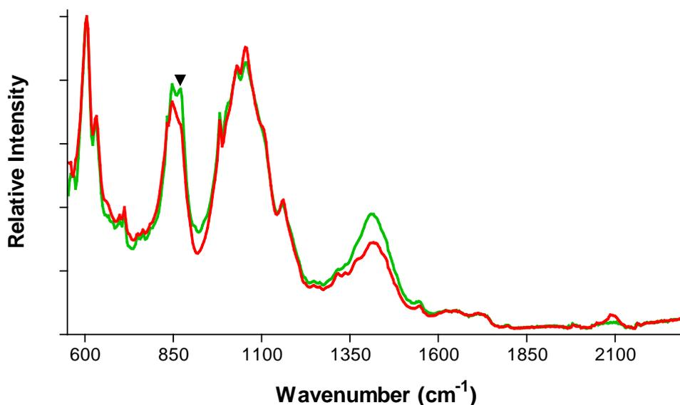
FTIR spectrum in the fingerprint region of the red-inked portion of the PSAG-585693 stamp (red trace) showing the NON-equivalence in spectrum with that of the red-inked region from the **C23c** reference spectrum (green trace). The diagnostic chrome red peak at 870 wavenumbers characteristic of the C23c stamp is marked with the solid wedge symbol.
