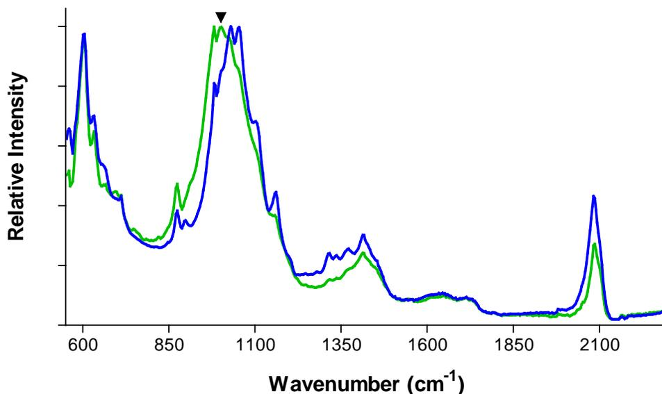
FTIR spectrum in the fingerprint region of the blue-inked portion of the PSAG-585693 stamp (blue trace) showing the NON-equivalence in spectrum with that of the blue-inked region from the **C23c** reference spectrum (green trace). The diagnostic ultramarine peak at 1001 wavenumbers characteristic of the C23c stamp is marked with the solid wedge symbol.
