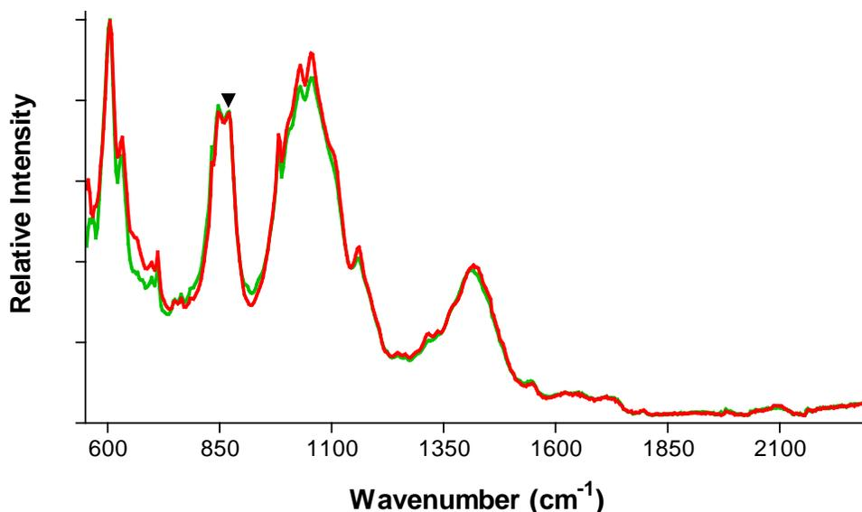
FTIR spectrum in the fingerprint region of the red-inked portion of the PSAG-585693 stamp (red trace) showing the equivalence in spectrum with that of the red-inked region from the **C23c** reference spectrum (green trace). The diagnostic chrome red peak at 870 wavenumbers characteristic of the C23c stamp is marked with the solid wedge symbol.
